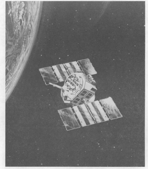
SANDIA PROVIDED Nuclear Detonation Detection System payloads for the four Global Positioning System satellites (one is shown in this drawing) launched last year.
